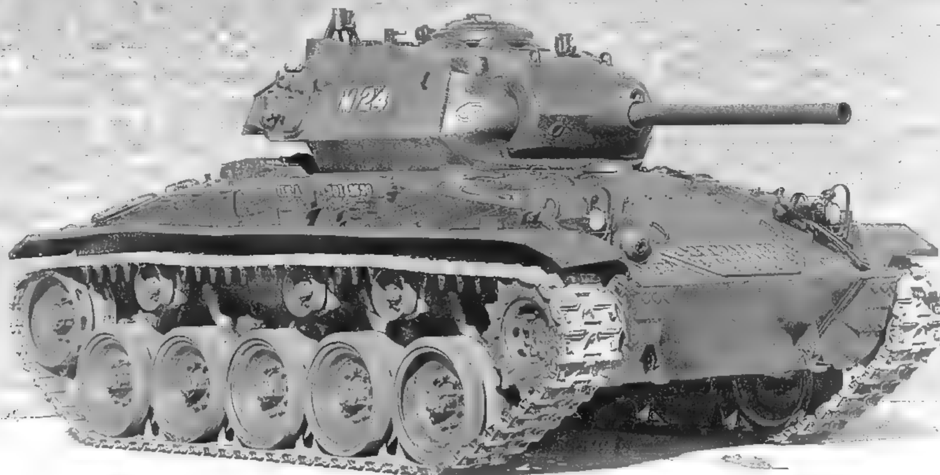
In this official Armor and Engineer Board portrait of the M24, the road wheel arrangement associated with U.S. tank torsion bar suspension is illustrated. This type of suspension would be used on virtually all subsequent U.S. tanks. (Photo courtesy of Patton Museum)
